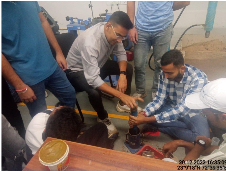
Fig: Explanation of Proctor Compaction Test
